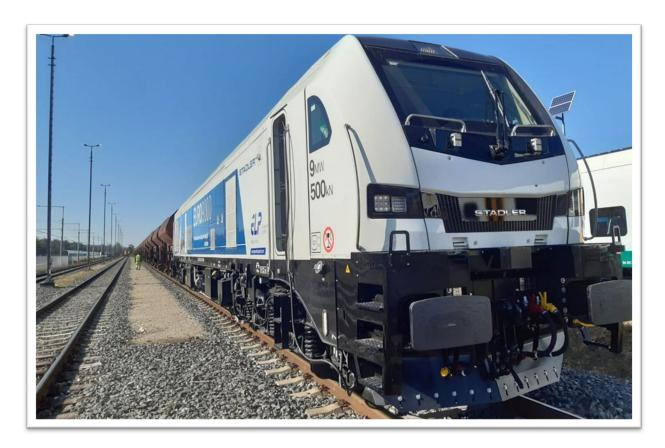
The EURO9000 is the new Hybrid multi-system locomotive for use throughout Europe. The locomotive enables up to 500kN tractive effort with an output of 1.9MW in diesel mode and up to 9MW in electrical mode. The Euro9000 platform is natural evolution of Stadler's successful EuroDual and Euro4000 locomotive family.
