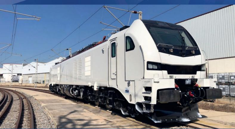
The new EuroDual six-axle hybrid locomotive is more than just a locomotive for the "last mile" and offers two solutions in one. It can be used for heavy-haul operations on both electrified and non-electrified lines. During operation, it is possible to switch from the electric to diesel mode.
