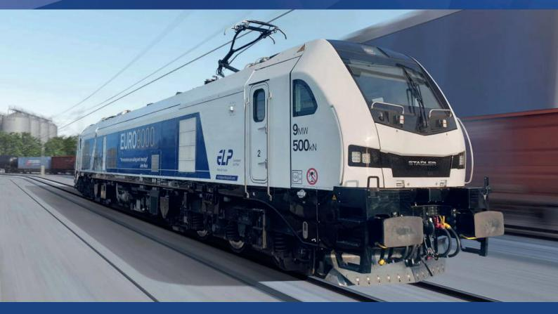
The EURO9000 is a next-generation hybrid multi-system locomotive for use throughout Europe, combining efficiency with flexibility. The locomotive enables up to 500 kN tractive effort, with an output of 1.9 MW (2 x 950 kW) in diesel mode and up to 9 MW in electrical mode. The Euro9000 platform is an evolution of Stadler's successful EuroDual and Euro4000 locomotive platforms.
